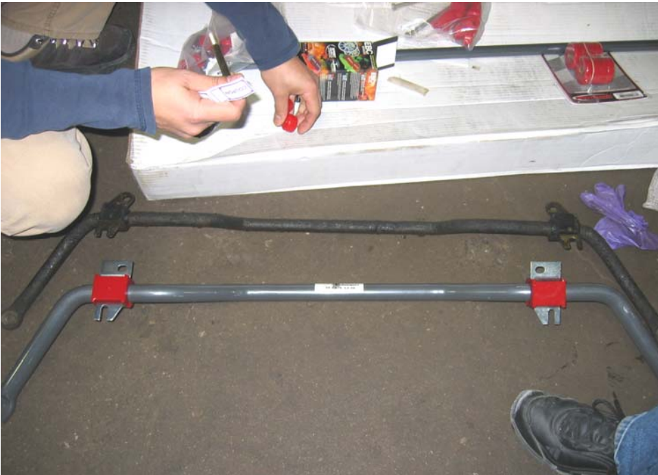
Stock sway bar vs Suspension Techniques sway bar, big difference, 66% increase in cross-section area
