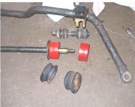
New polyurethane bushings installed on tension/compression rod
