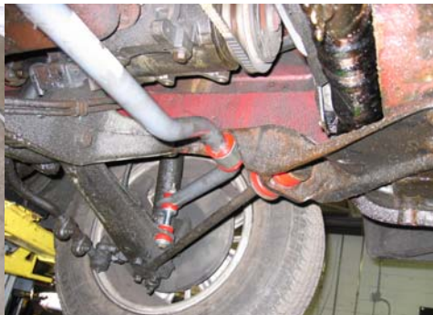
New beefy front sway bar & bushings installed
