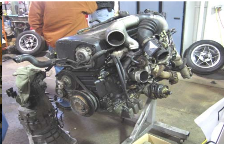
Skyline GTR motor being prepared to be transplanted
